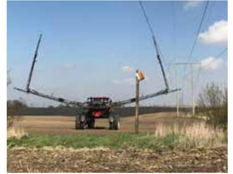
If equipment comes into contact with a power line, assume the line is energized and deadly. The operator should NOT get off the machinery unless in immediate danger. If the operator touches the ground and the equipment at the same time, they will become a channel for electricity. Instead, the operator should stay on the equipment and contact the local electric utility or 911 immediately to report the incident so power lines can be deenergized safely before exiting. ⚡
