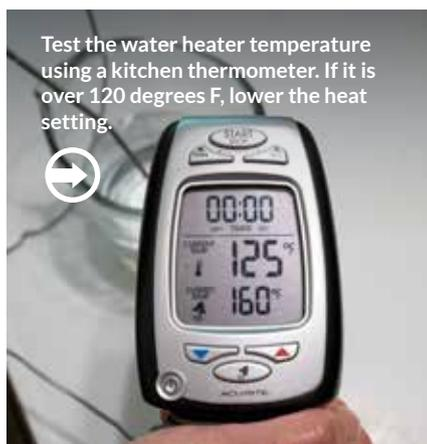
Test the water heater temperature using a kitchen thermometer. If it is over 120 degrees F, lower the heat setting.
